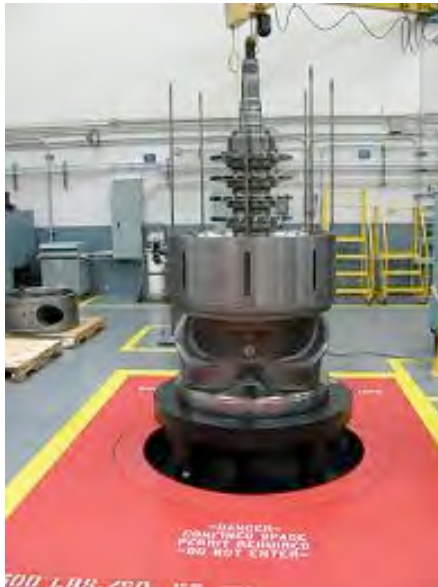
Figure 6.6 Installation of rotor into inlet system
