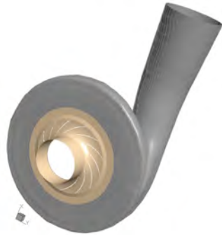
Figure 1.20 Coupled analysis: impeller, diffuser and volute grid
