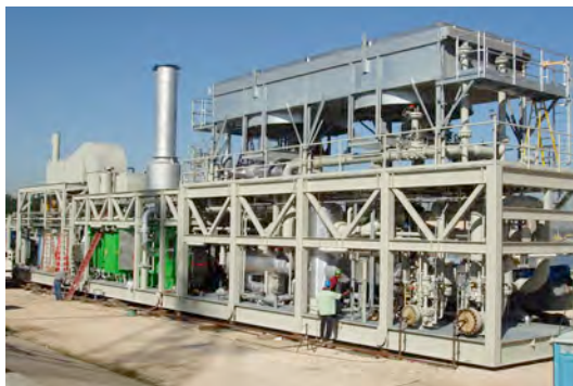
Figure 11.4 Process module and control room
