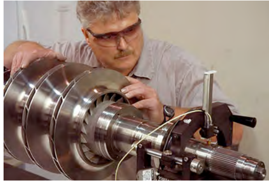
Figure 6.2 Inspecting impellers during restage at Solar's Mabank facility
