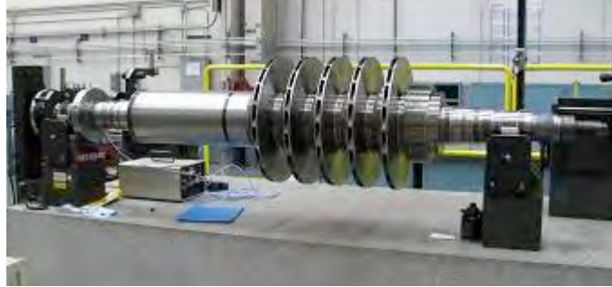
Figure 6.5 Electro-mechanical run-out checks
