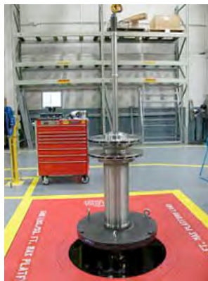
Figure 6.3 Rotor assembly in build pit
