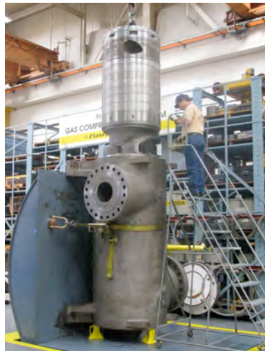
Figure 6.12 Vertical module installation
