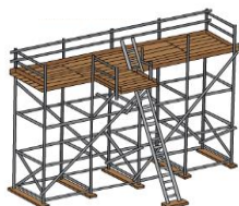
Tube and Coupler Scaffolding
