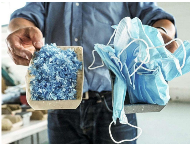
Figure 6.44 Shredded PP facemasks (Source: https://recyclinginternational.com/gallery/plaxtil-puts-single-use-face-masks-back-in-the-loop/32591/ ).
