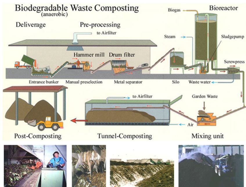
Figure 10.24 Industrial composting process (Source: Yip & Madl, 2003).
