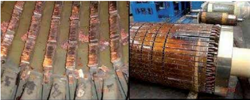
Figure 26. Stator and Rotor Damages
