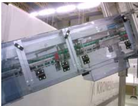
Preform conveyor covered to protect from contamination
