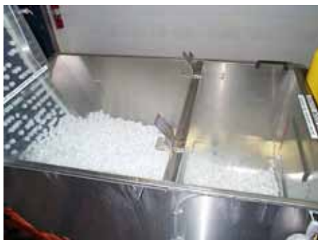
Cap delivery system hygienically covered
