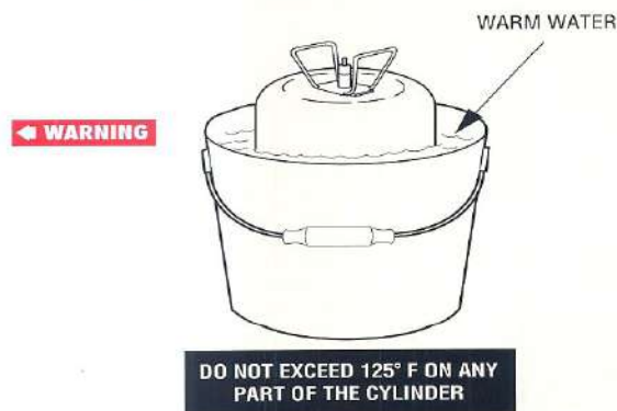
▼ Figure 2-12. Warming Cylinder with Warm Water
