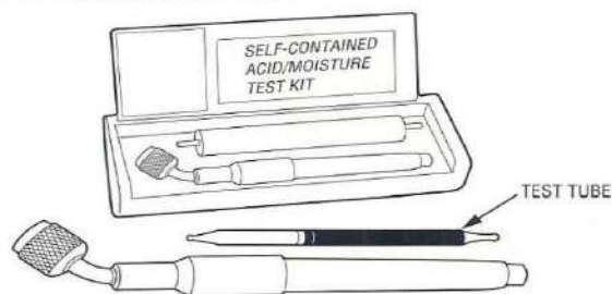
▼ Figure 1-20. Self-Contained Acid/Moisture Test Kit
