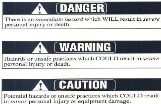
▼ Figure 2-23. Typical Terms Used to Prioritize Safety Hazards
