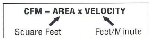
▼ Figure SP-16-1. How to Calculate Airflow
