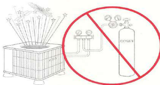
▼ Figure 2-16. Oxygen Mixed with Oil can Cause an Explosion
