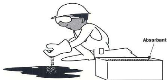
▼ Figure 2-19. Always Clean Up Oil Leaks Immediately
