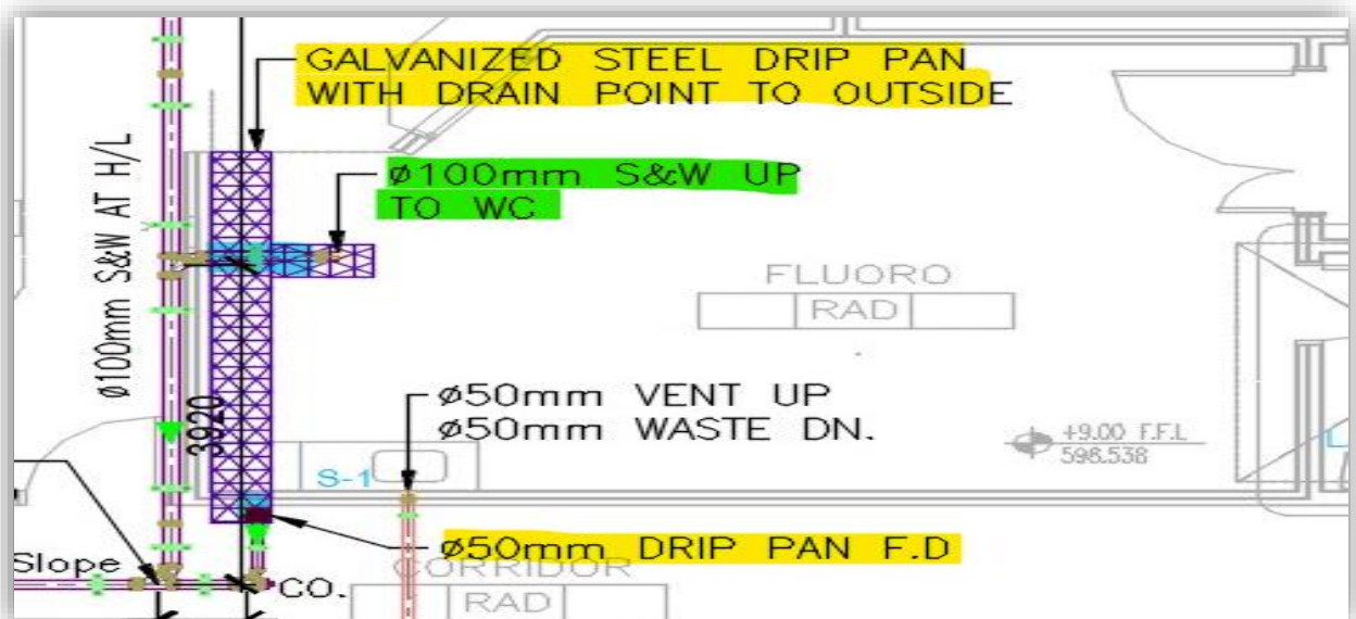
Drip Pan photo from Construction Drawing
