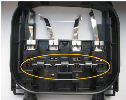
Figure 25: Bypass Diodes Are Typically Located in Module Junction Boxes
