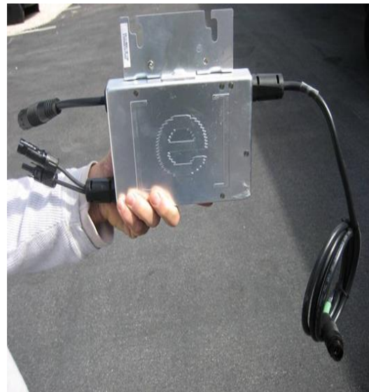
Figure 32: Micro Inverters Are Installed Adjacent to Individual PV Modules
