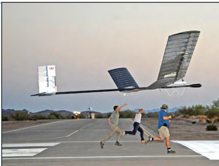
The solar-powered Zephyr can stay in the air for days at a time.
