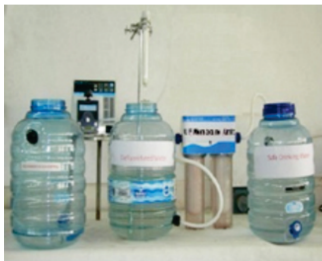
Figure 54: BARC De-fluoridation Unit
