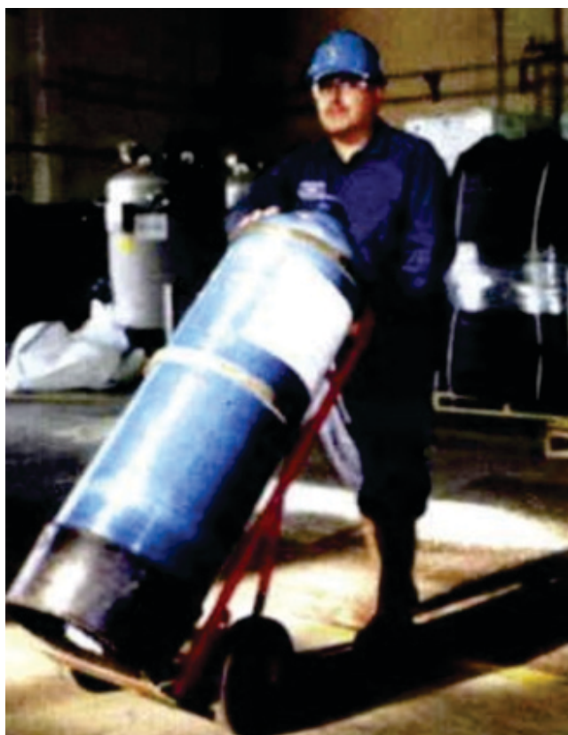
Figure 94: Siemens Ion Exchange Resin Canister
