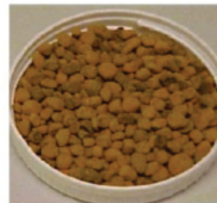
Iron oxide coated sand Source: UNESCO-IHE
