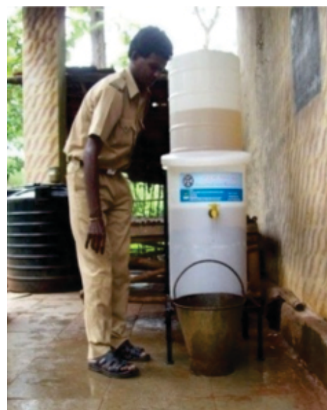
Figure 57: Household Iron Removal - CSIR - NEERI Technology
