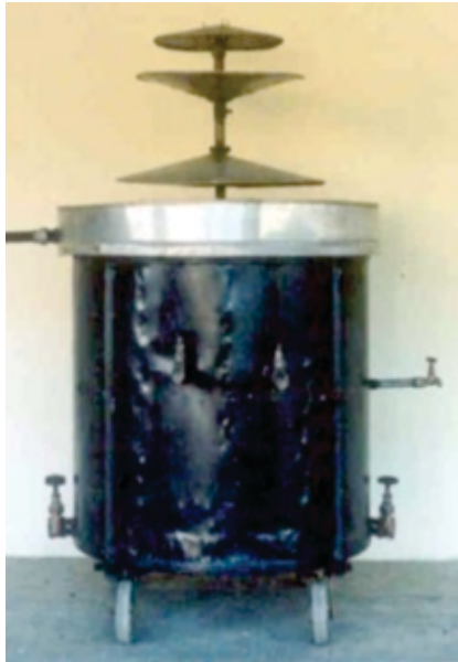
Figure 61: Water Iron Removal Unit of DRDO
