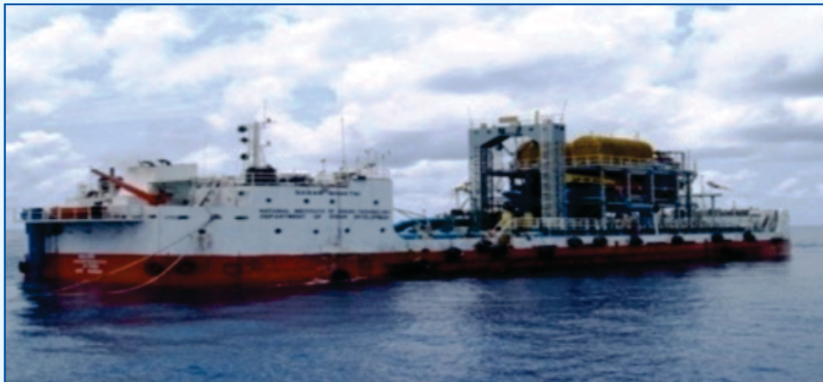
Figure 83: Details of the barge mounted 1 MLD Demonstration LTTD plant
