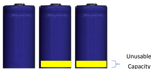
Figure 6 Imbalanced cells at end of discharge.
