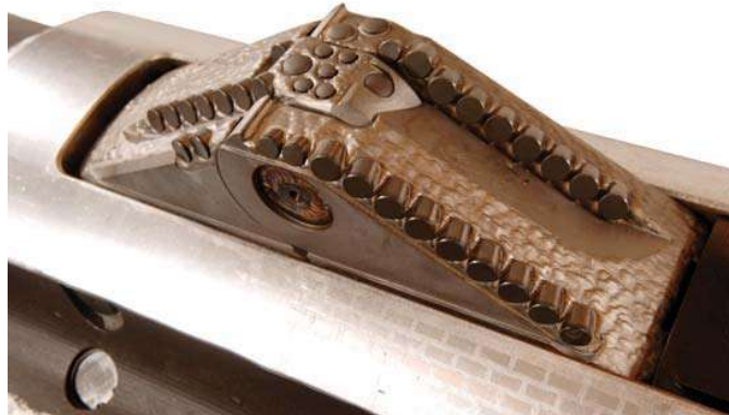
C-5 Halliburton under-reamer
