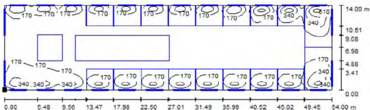
Figure 51. Daylighting simulation results for illuminance on a 80 cm high plan over the floorplan, for a clear sky day at 10.30 a.m.
