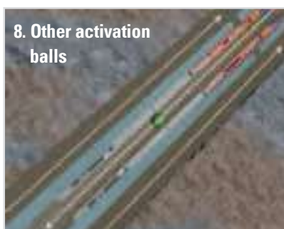
8. Other activation balls Other ball activation tools that use smaller diameter balls can be positioned below the WELL COMMANDER tool as the ball will not activate it
