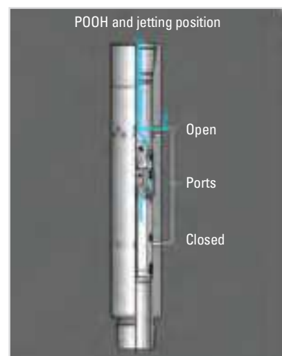
Figure 2. The upper ports can be opened by dropping a second ball and applying pressure.
