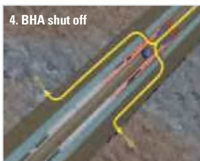
4. BHA shut off Optional shut-off ball can be landed on lower ball seat to prevent LCM or WSM from entering the BHA while treating the formation
