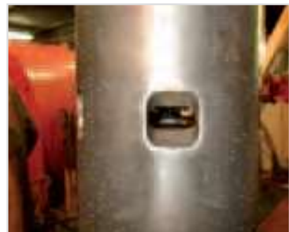
Open circulating ports provide generous flow area
