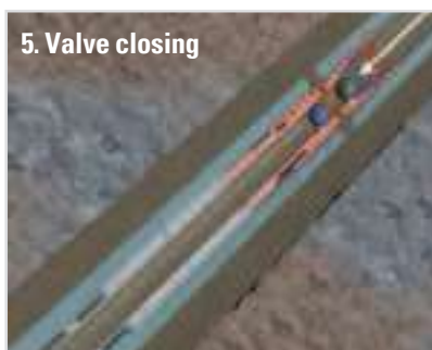
5. Valve closing The BHA shut-off ball is removed when subsequent activation ball closes the ports
