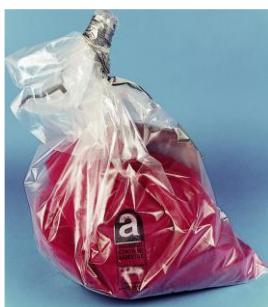
Figure 7.12.8: Asbestos Waste - Double Bagged
