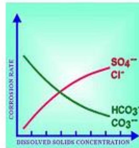
Dissolved solids other than alkalinity influence corrosion based on the following factors: aggressive chloride and sulfate ions can destroy the protective oxide layer on the metal surface; the greater the concentration of aggressive ions, the faster corrosion occurs. Also ions can concentrate under deposits to form localized corrosion. The greater the concentration of aggressive ions present in solution, the more rapidly corrosion proceeds.
