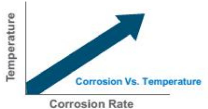
Increases in temperature and oxygen will usually increase the rate of most corrosion reactions. As a rule, each 18 degrees Fahrenheit increase in temperature doubles the rate of most chemical reactions. As the temperature increases, the cathodic reaction proceeds faster, and the oxygen diffusion rate improves. Click the button to view the results of this process.
