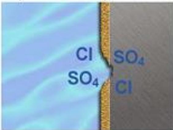
Ions can concentrate under deposits to form localized corrosion.
