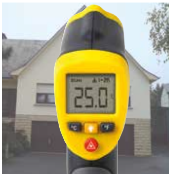
IR thermometer, temperature measurement in one spot
