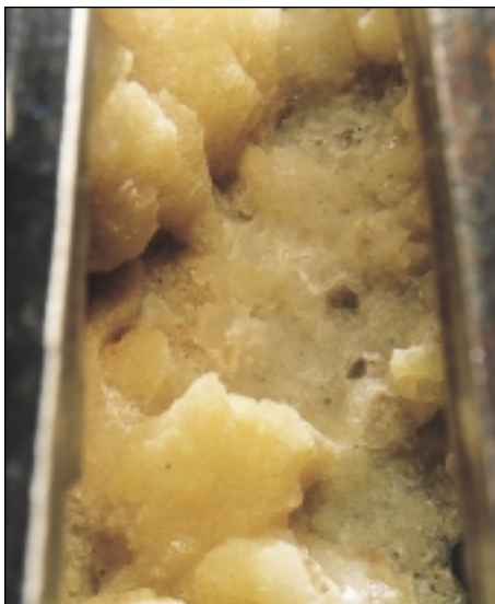
▲ Removing calcium carbonate scale with water jetting. The tubing was jetted with a single water jet at a rate of 2.4 in./min [1 mm/sec]. Although carbonate scale has been removed, a considerable amount remains in place.
