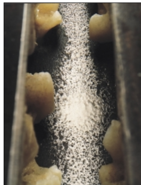
▲Tubing scale removed with the Sterling Beads abrasive. The tubing was jetted with Sterling Beads abrasive in a single water jet at a rate of 2.4 in./min [1 mm/sec], to remove carbonate. During the test, the jet was held stationary for 3 minutes, and less than 2% of the steel was removed from the tubing wall.
