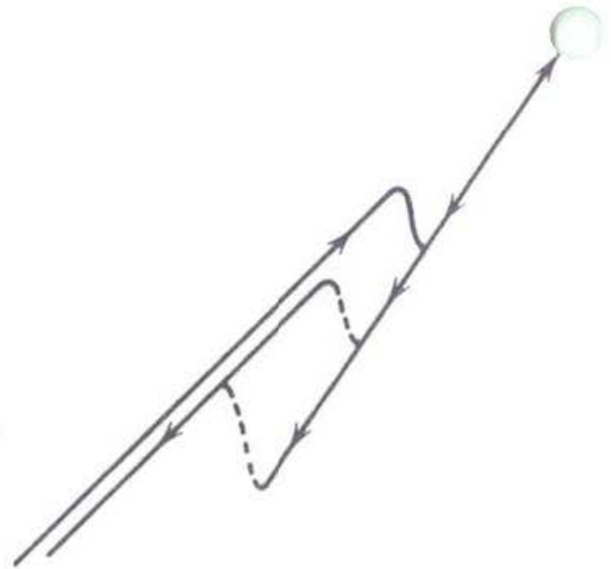
Schematic presentation of the expansion of a low-carbon steel during heating and
