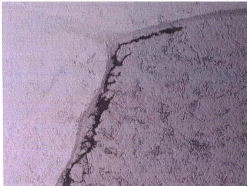
nipple-tube weld cross-section. Creep damage. Magnification 100x. Nital etched. Stainless steel weld metal on Cr. 2 (T22)
