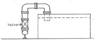
5. A cross connection to a sprinkler system can cause back siphonage when a partial vacuum in the water system draws water from pooled water near a sprinkler head. This type of cross connection led to the "Holy Cross Episode" that was mentioned earlier. Backflow caused by back pressure can occur when the sprinkler head is at a higher elevation than the connection to the potable water system.
