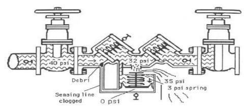
RPZ with Clogged Sensing Line with 0 psi in the Sensing Line. The pressure inside the zone is 32 psi, and the pressure acting to open the relief valve is 35 psi. If the sensing line is clogged and the pressure acting to keep the relief valve closed is 0 psi, the relief valve will open and continue to dump water from the zone until the sensing line is cleared allowing water pressure to the upstream side of the diaphragm.
