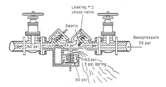
RPZ Failing Second Check Valve during Back Pressure Conditions. If a pump connected to the consumer's potable water line creates a pressure of 59 psi and the second check valve is leaking, the pressure acting to open the relief valve is 62 psi (59 psi + 3 psi), while the pressure acting to keep it closed is only 60 psi. Therefore, the relief valve will open.
