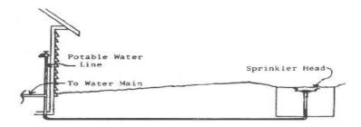
6. A cross connection to a pressurized pipe carrying contaminated water can cause backflow. When the valve is opened, backflow by back pressure can occur if the pressure in the non-potable lines is higher than the positive pressure in the potable system.
