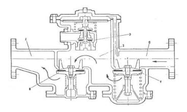
NOTE: The RPZ above must be accompanied by a valve on both ends to be an approved and testable RPZ assembly.
