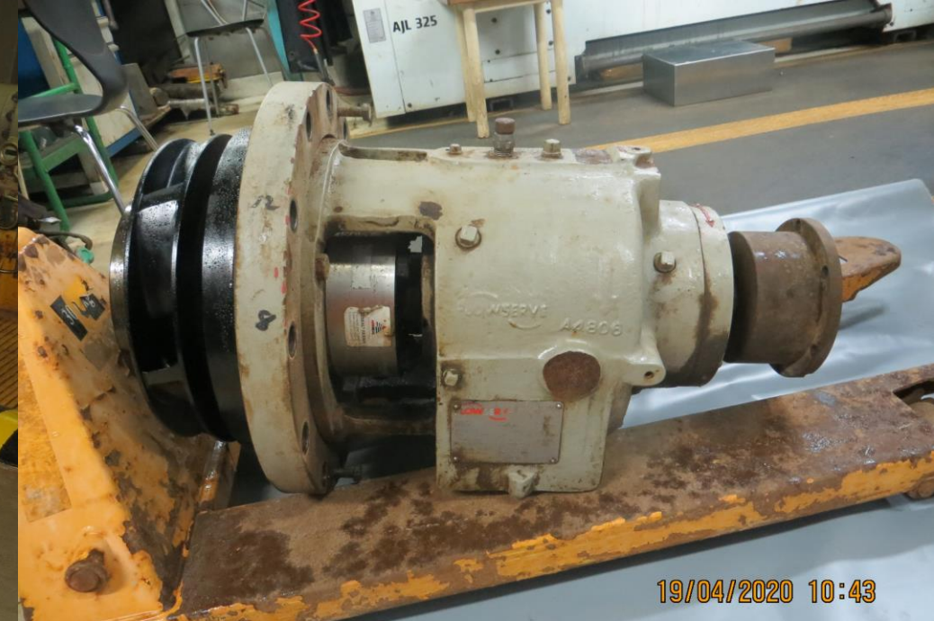
API OH2 Crude oil export pump picture
