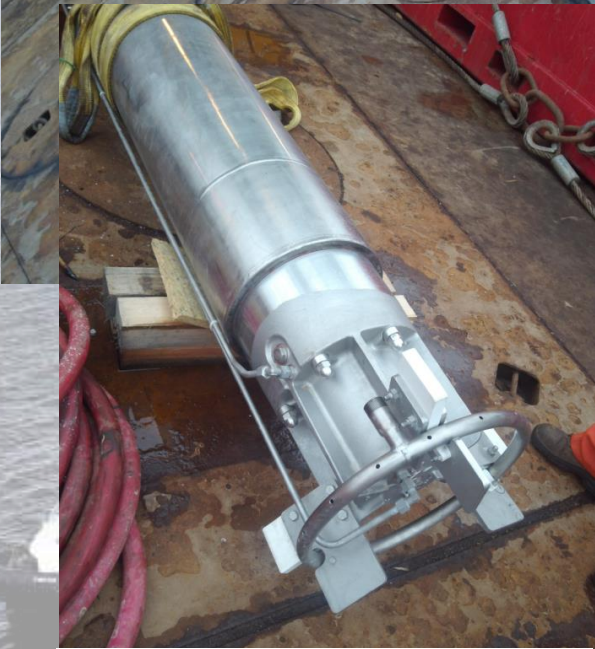
Sea water lift pump picture
