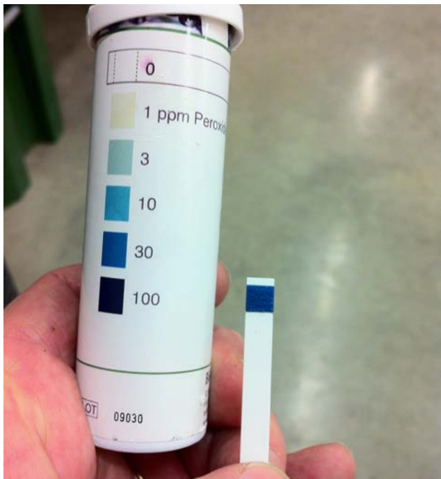
Figure 43. Colorimetric test strip for hydrogen peroxide concentration.
