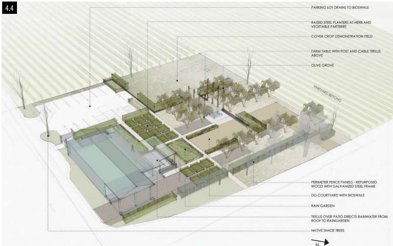
Figure 4.4 A diagram of the stormwater management strategies of the landscape.
