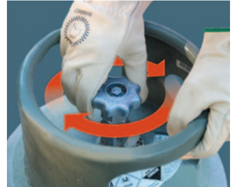
Ensure cylinder valve is closed before moving or disconnecting equipment
