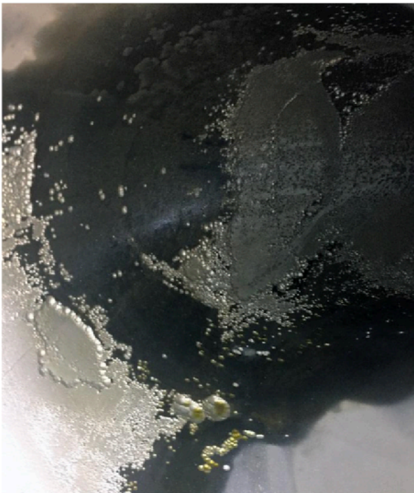
Figure 1: The left image shows a pitted and cratered pipe surface. The right image shows a material that has corroded since being removed from service, contaminating the surface, and making analysis of the original cause of pitting difficult.
