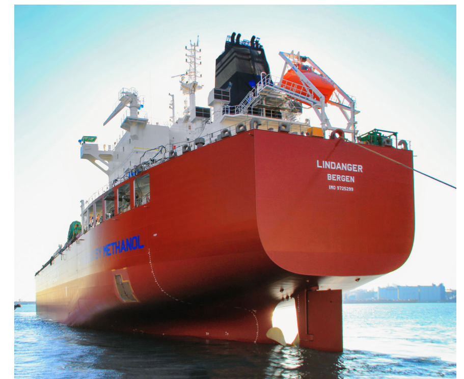
Lindanger, the world's first dual-fuel, methanol-ready tanker, was built in 2016 to DNV class.
