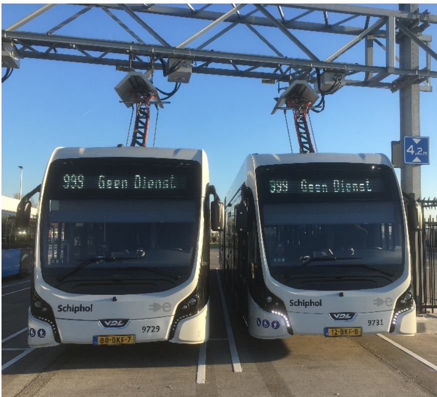
Opportunity charging of busses using a pantograph (photo: DNV)
