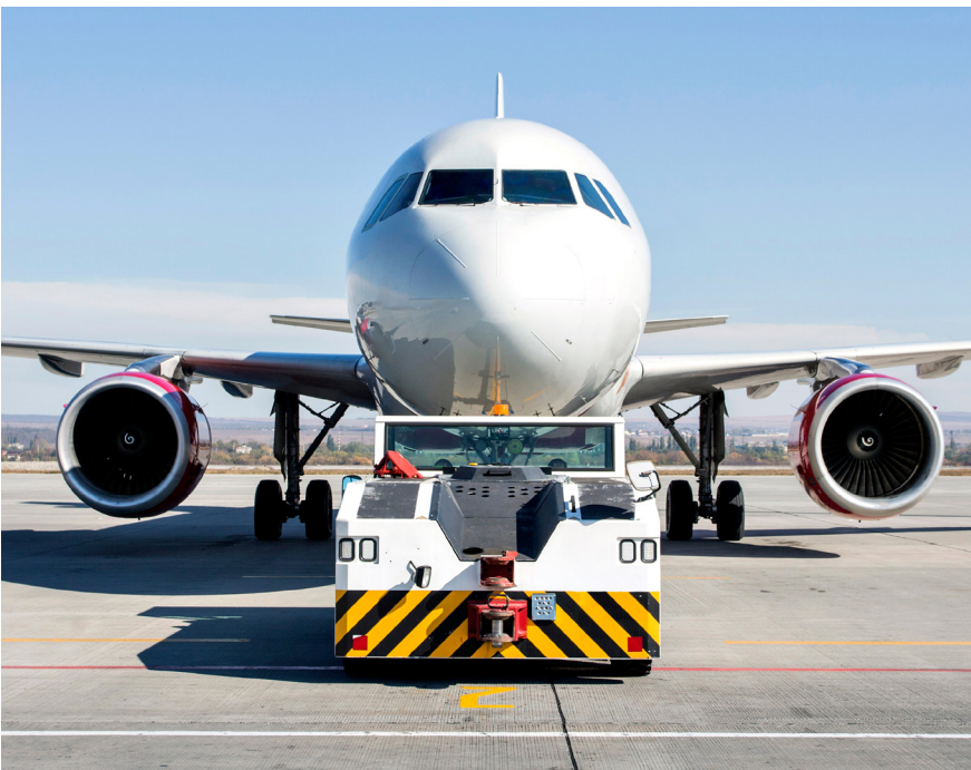
FIGURE 3.19 Electric towing could lead to average fuel savings of 8%
