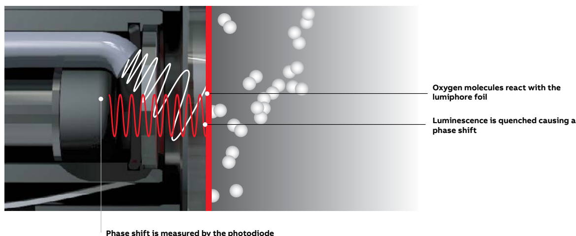
Figure 6 Optical sensors – how they work
