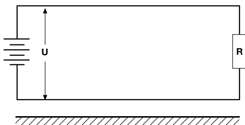
Figure 9 Network insulated from earth
