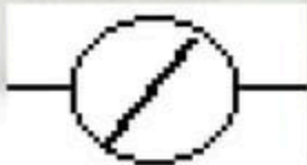
An OUT Bar (normally closed coil) symbol
