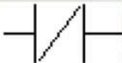
A Load Bar (normally closed contact) symbol
