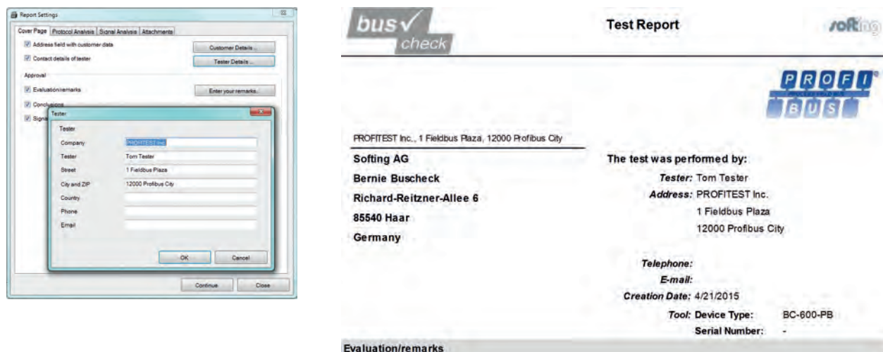
Figure 12: Detailed Test Report Summarizing the Results of a PROFIBUS Network Acceptance Test
