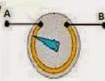
Connections For Fixed resistance
