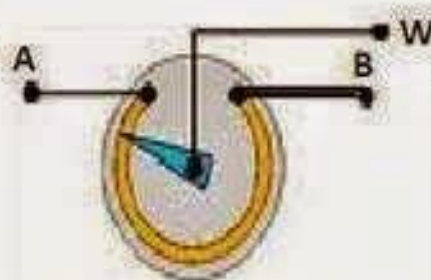
Connections For voltage division
