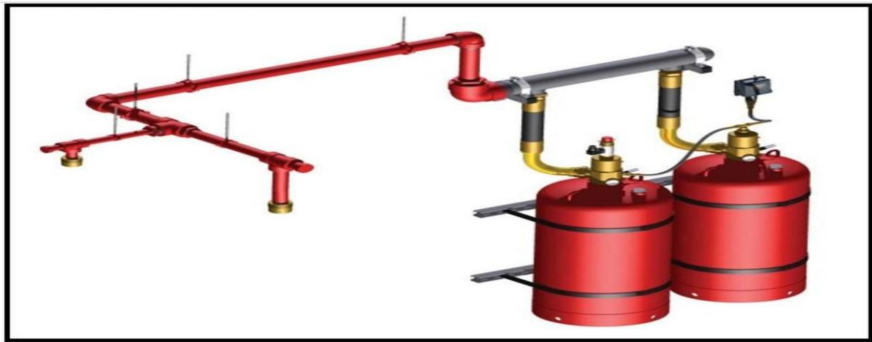
**Distribution** Pipes must be made of non-combustible materials, Pipe shall be of material having physical and chemical characteristics such that its integrity under stress can be predicted with reliability. Special corrosion-resistant materials or coatings shall be required in severely corrosive atmospheres.
