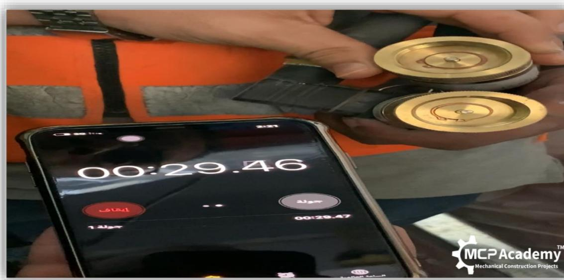
Ensure the periods and duration of delays in the system, where the alarms are activated from the smoke sensors in the system, and start testing the performance of the electric operating valve that is installed on the actuator cylinder head.
