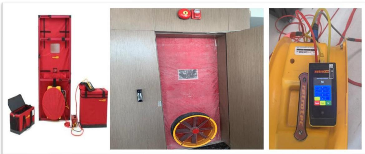
The devices shown in the picture are used to pressurized the room, obtain readings, then release the room from depressurized room air, and compare the readings to ensure that there are accepted reding for air leaks so that not to release gas outside the room case of fire
