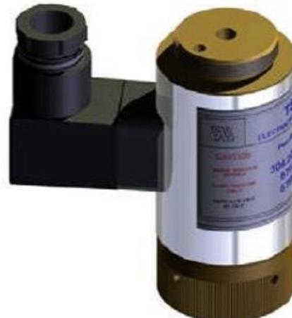
An electric actuator is a Solenoid Valve that takes a signal from the control panel to allow gas to pass at the time of the fire. It is used as a primary means of automatic activation of the system and is provided with a part for manual activation.
