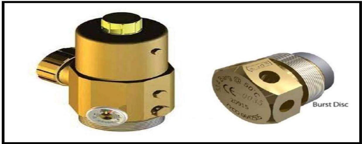
**Safety Relief - Burst Disc** A safety switch that works to discharge excess pressure from the cylinder when the gas pressure inside it is increased in cases of high temperature in order to avoid an explosion in the cylinder
