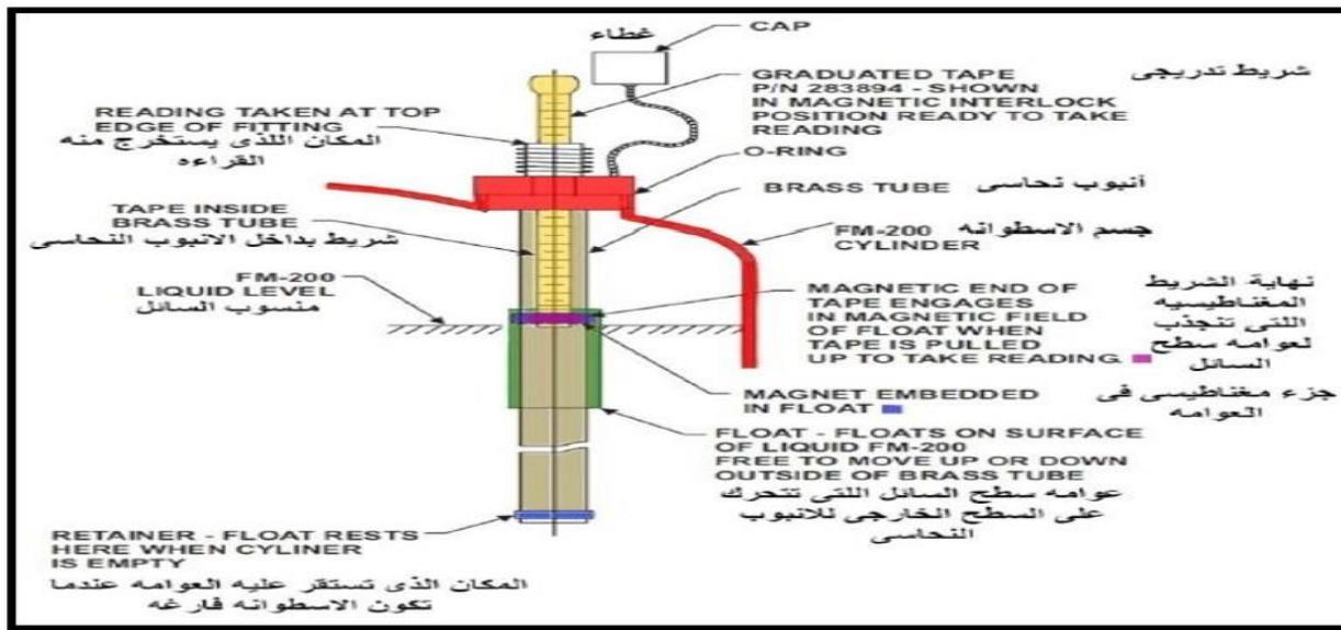
the indicator of the level of the liquid in the cylinder is used in the periodic inspection of the content of the cylinder, where the level of the liquid is an indicator of the amount of liquid inside the cylinder
