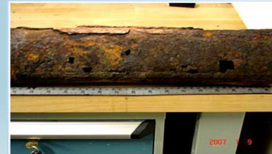
Corrosion damage seen on pipe
