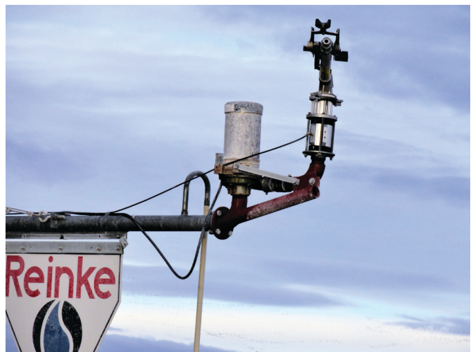
Figure 63. Example of a centrifugal pump used to boost pressure for the end gun of a pivot.
