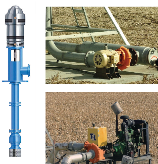
Figure 75. Examples of direct drives for motors and engines (drawing is courtesy of ITT Gould Pumps).
