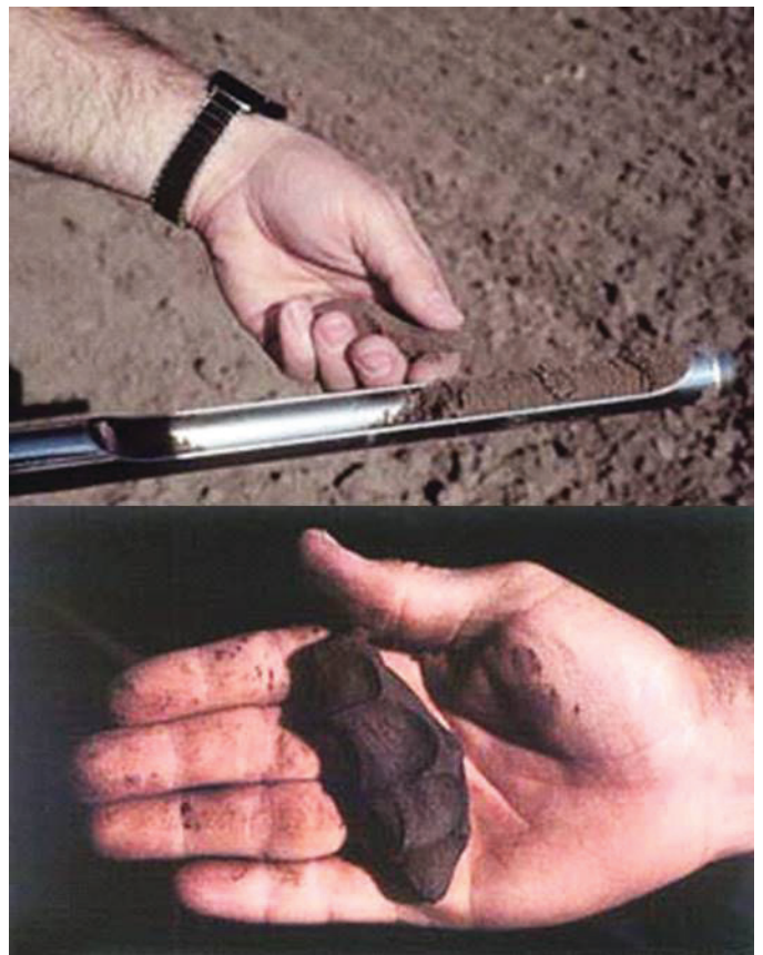
Figure 31. Sampling and evaluation techniques for the feel method of soil water monitoring.
