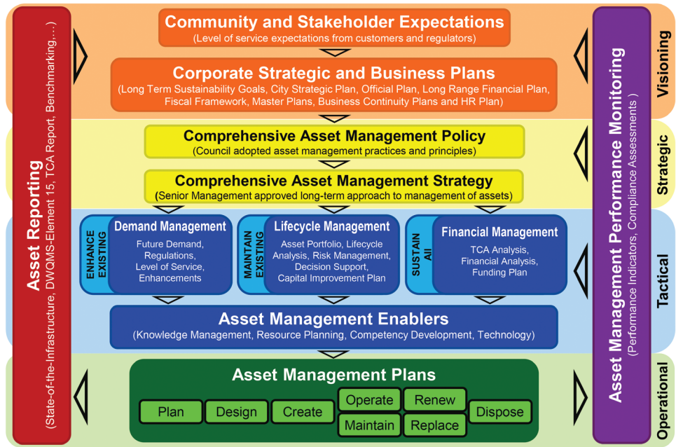
Figure 3.4: City of Ottawa Comprehensive Asset Management Framework
