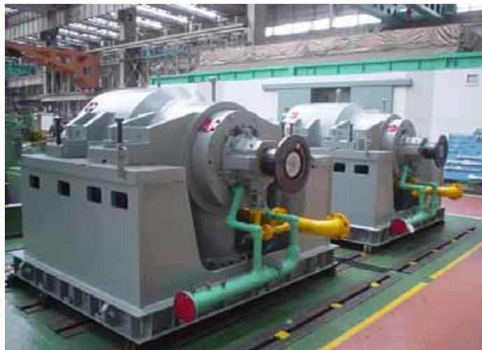
Boiler Feed Pumps for Zouxian Power Plant
