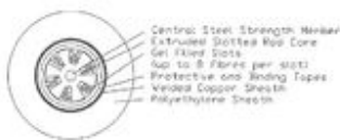
Composite subsea power and fibre optic cable
