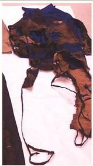
Damage caused by arc faults
