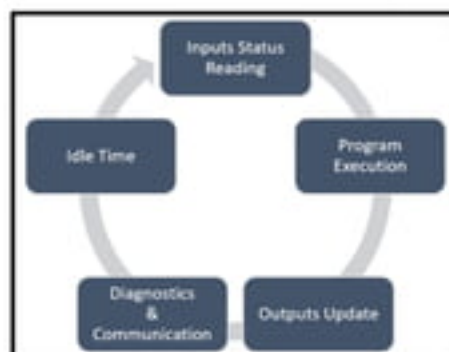
Figure 13: Programmable Controller Total Scan Cycle Representation
