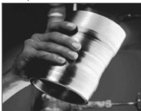
Figure 2.23 – Wear on Shaft/Sleeve Due to Tight Packing
