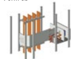
Structural frame of a compartment with moulded-case circuit-breaker in form 3b
