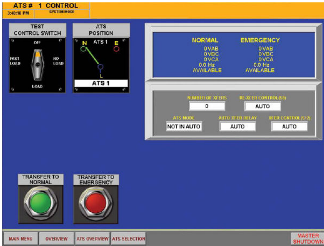
Figure 10 – ATS Remote Monitoring Software Screens
