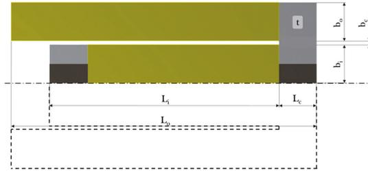
**Figure 18.** Parameterization of the reference geometry (light grey corresponds to steel, black to NdFeB, and yellow to PIC255).
