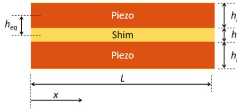
Figure 2. Cross-section of the piezoelectric bimorph beam.
