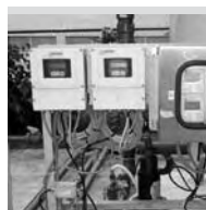
EMF with remote electronics
