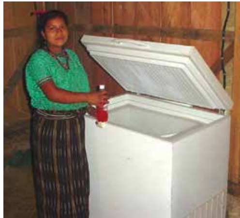
Fig. 12. SunDanzer PV direct drive refrigerator piloted in the indigenous Mayan village of Santa Clara, Quiché, Guatemala by NMSU, NASA, and Fundación Solar in 2002.
