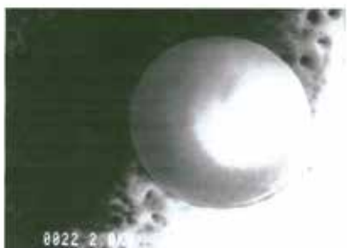
3a. Spherical particle. Main elemental composition: Mg, Si, O (traces Ca, Fe). The morphology of the particle indicates that it once was in a realm where the temperature was higher than its melting temperature. Another possibility would be the emission from a melt.
