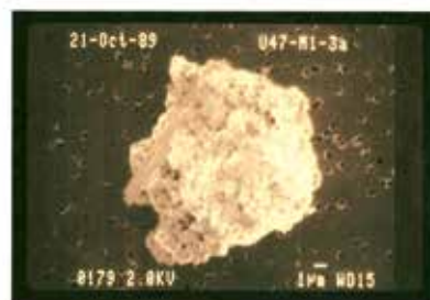
3b. This particle seems to be a conglomerate of smaller particles. Main elemental components: Mg, O (N, C, H).
