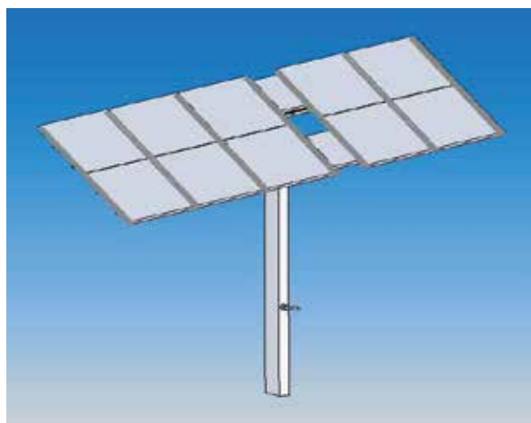
Fig. 2. The 3KW polar-axis solar power platform
