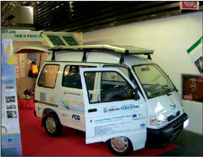
Fig. 10. A prototype of Hybrid Solar Vehicle with series structure developed at the University of Salerno.
