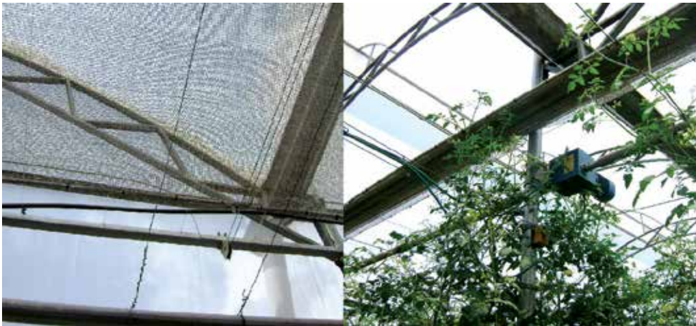
Fig. 8. Elements used for closing and opening the shade curtain including gear motor, pulleys and Raschel net.
