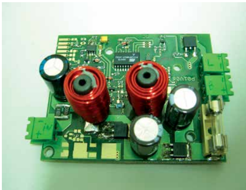
Fig. 9. Photo of the MPPT and battery charger prototype board.
