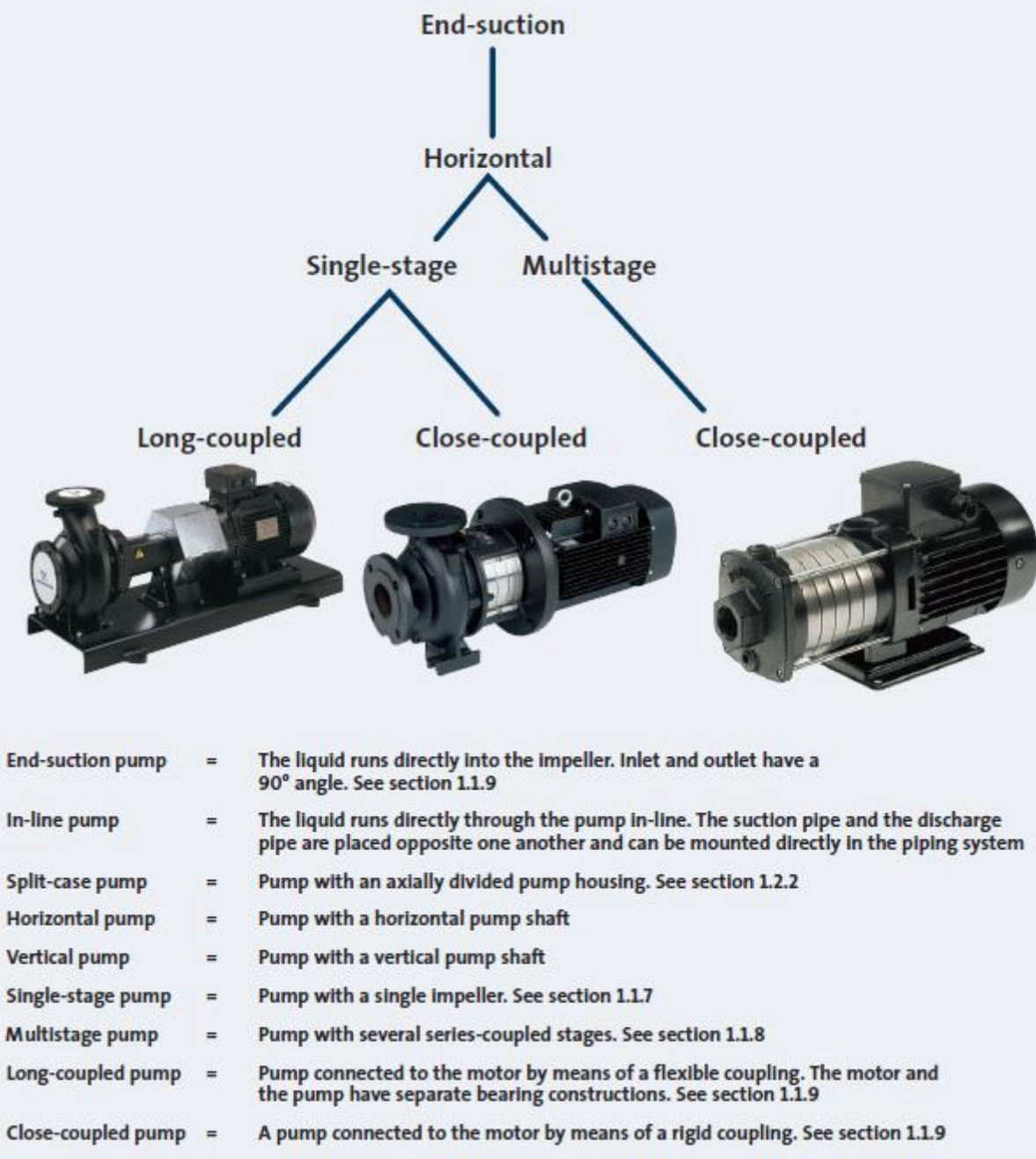
fig-13. most end-suction and in-line pump types
