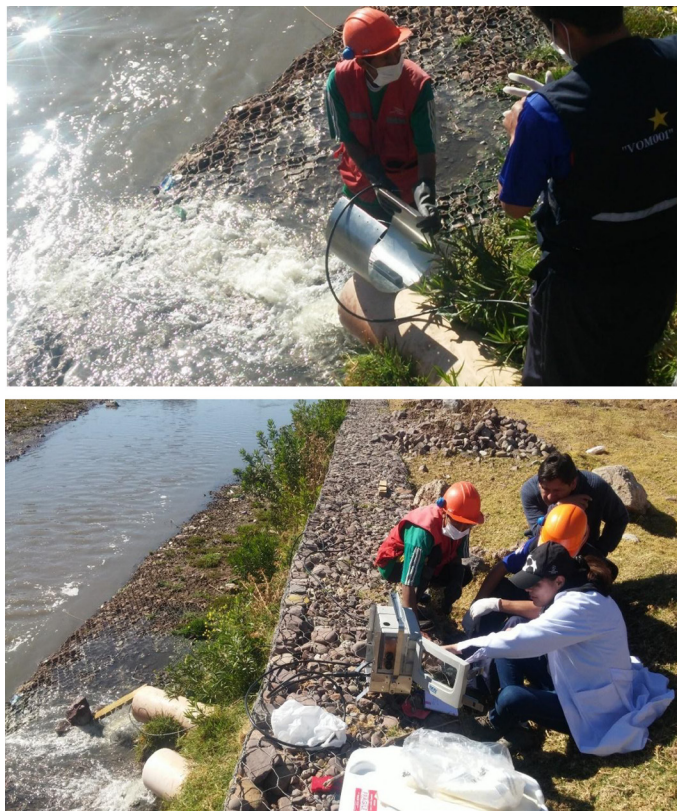
Figure 3.12 Measuring flowrate with an area velocity digital flow meter, which has ring inserts for different diameter sewers, for the design of a wastewater treatment plant for a small city, Saylla, Peru. Note the second discharge pipe that was not part of the original sewer design and was clandestinely added more recently as a result of rapid population growth. Photos courtesy of CONASIN SRL, Cusco, Peru.
