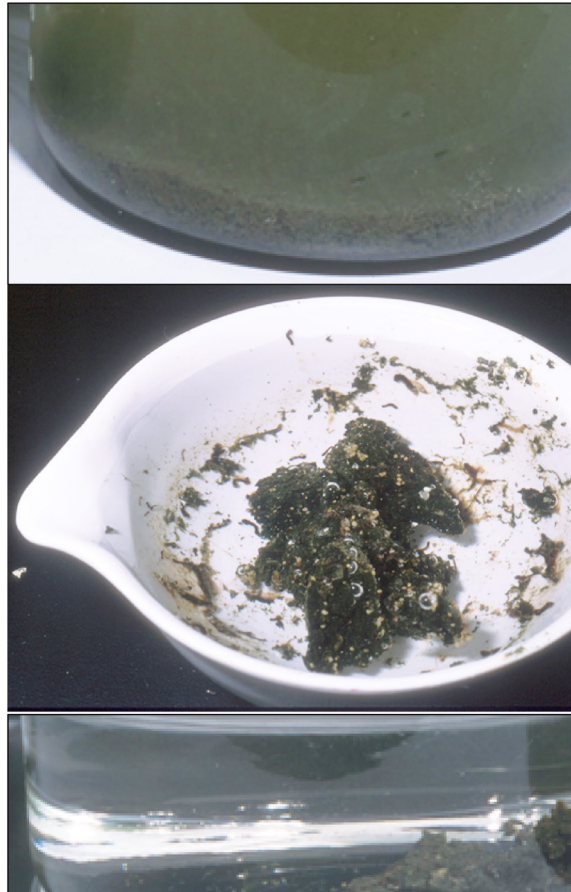
Figure 6.20 Top photo: A beaker of settled algae from the Biggs pond effluent. Middle photo: Air-dried algae in a crucible that was filled with algae from the top beaker. Bottom photo: The air-dried algae does not rehydrate when placed in a beaker of water.
