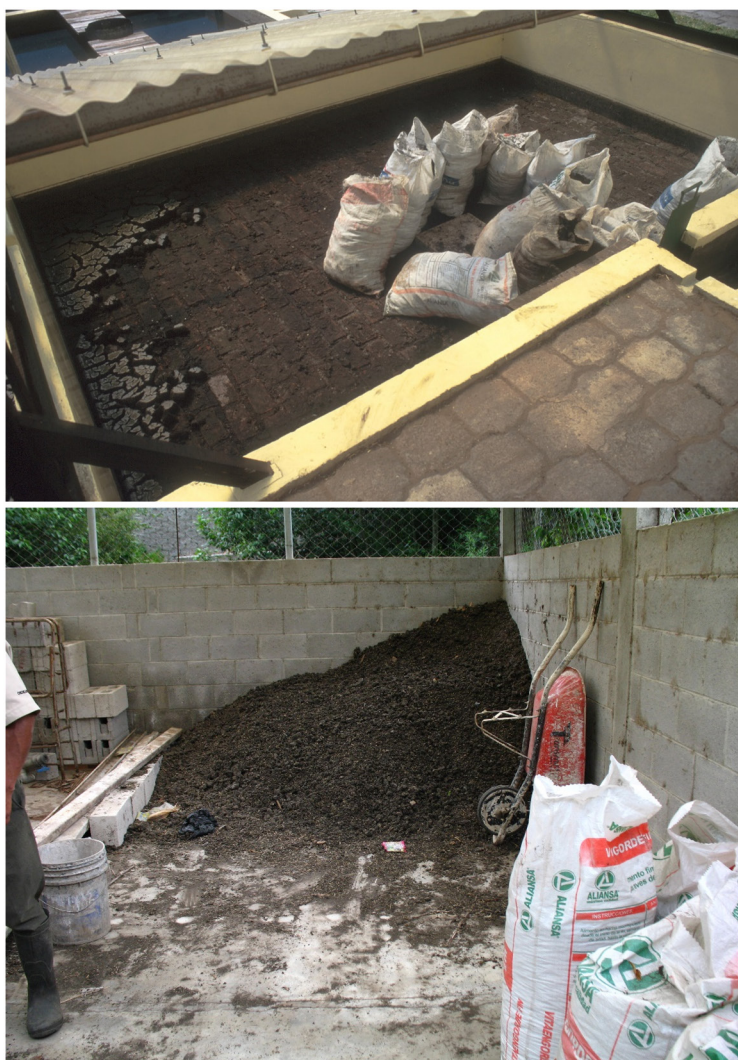
Figure 7.6 Dewatered UASB sludges from two small treatment plants in Guatemala are distributed in bags to give to the local population as a fertilizer and a soil conditioner. This is a common practice in many small cities that should be prohibited: A significant fraction of all influent pathogens will concentrate in the sludge. As an example, concentrations of helminth eggs in UASB sludges have been reported up to 62.9 eggs/g dry weight (Oakley et al. , 2017). The prevalence of soil-transmitted helminth infections in Guatemala is >50% (Figure 7.3). These sludges should be well dried and buried onsite. (Top: Sololá; Bottom: Maria Tecún.)
