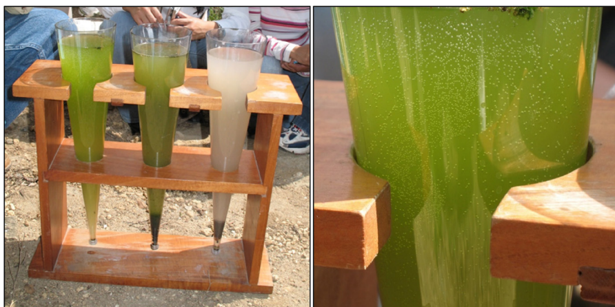
Figure 5.3 Algal growth in a well-functioning facultative/maturation pond system. The top photo shows, right to left, raw settled wastewater, settled facultative effluent, and settled maturation pond effluent. The facultative pond has high concentrations of algae that settle rapidly when confined to an Imhoff cone; the maturation pond effluent has lower concentrations that do not settle. The bottom photo shows oxygen bubbles formed as a result of supersaturation during photosynthesis. Dissolved oxygen concentrations can rise greater than 25 mg/L in facultative ponds, where the saturation concentration is 7–9 mg/L. (Aurora II Waste Stabilization Pond System, University of San Carlos, Guatemala.)
