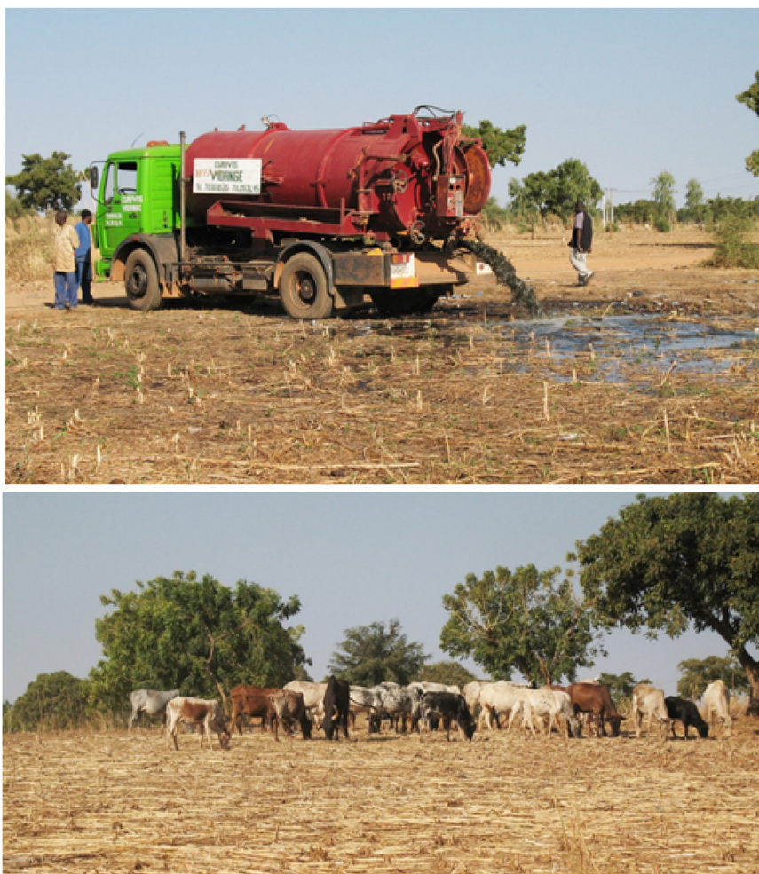
Figure 7.12 Disposal of liquid raw sludges from pumped septic tanks, latrines, and vault toilets, directly on agricultural lands in the outskirts of Ouagadougou, Burkina Faso. The grazing cattle are in the disposal areas used by the sludge haulers. As shown in Table 7.9 for Burkina Faso, the 4.75 \times 10^{-4} DALYs/ person yr for soil-transmitted helminth infections is 475 times greater than the WHO guideline of 10^{-6} DALYs/ person yr for reuse of sludge in agriculture. There are at least three fecal sludge treatment facilities in Ouagadougou developed to manage the serious treatment and disposal problem, but they are often overloaded and disposal directly on agricultural land is still common. Ouagadougou has a waste stabilization pond system designed for reuse in agriculture, but the majority of the population is not connected to the sewer system and still uses onsite systems for excreta disposal. The pond system is also one of the sludge treatment facilities, treating the leachate from fecal sludges deposited on drying beds adjacent to the WSP facility; the leachate is pumped to one of the anaerobic ponds designated for leachate treatment, while the dried sludges are permanently stored until analyses can be performed to determine if they are safe for reuse. Sludge treatment facilities are preferable to uncontrolled decentralized management of sludges.
