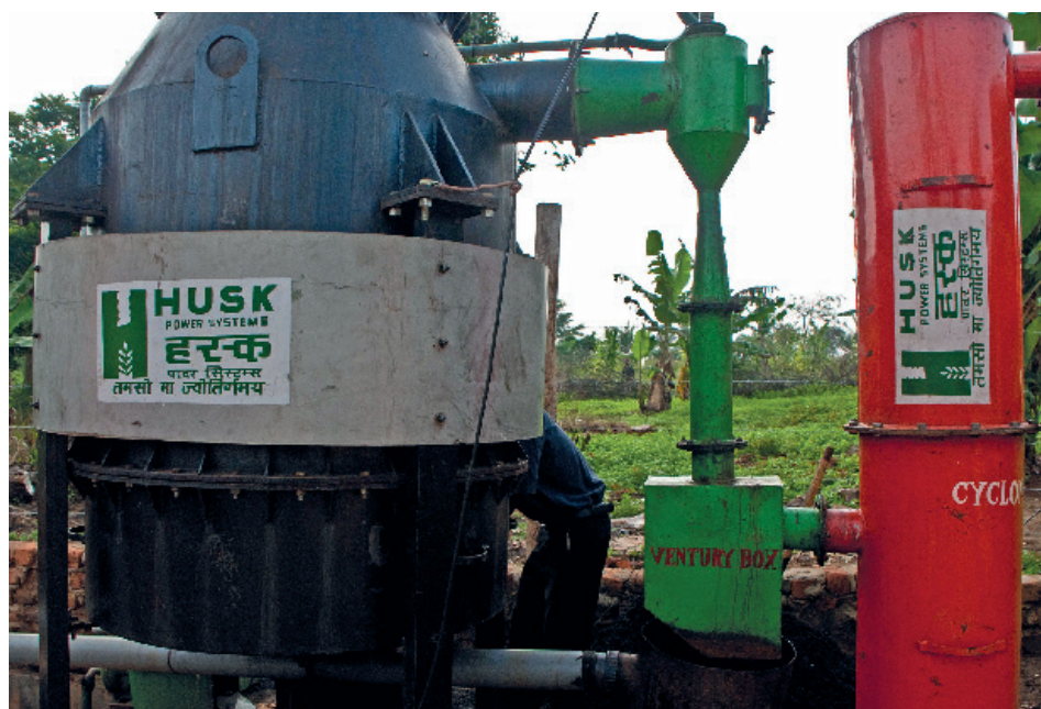
Figure 10.12 Iribogo gasification project utilising corn husks and sawdust, located in Muduma Sub-county, Mpigi District, Uganda (photo: Linda Strande).
