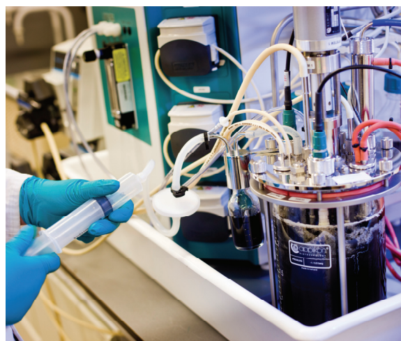
Figure 2.3.11 Collection of a liquid sample to determine the activity of sulphate-reducing bacteria (SRB). Note the characteristic black colour of the enriched SRB biomass in the reactor (photo: KWR Watercycle Research Institute, 2014).
