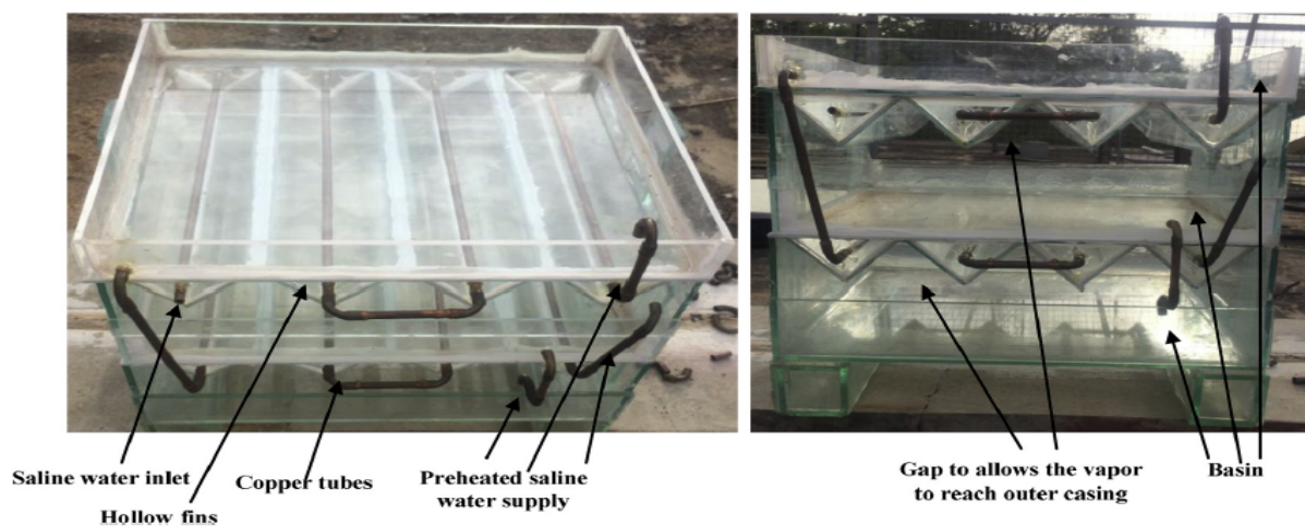
Figure 21. Photograph of a triple basin with triangular hollow fins [99].
