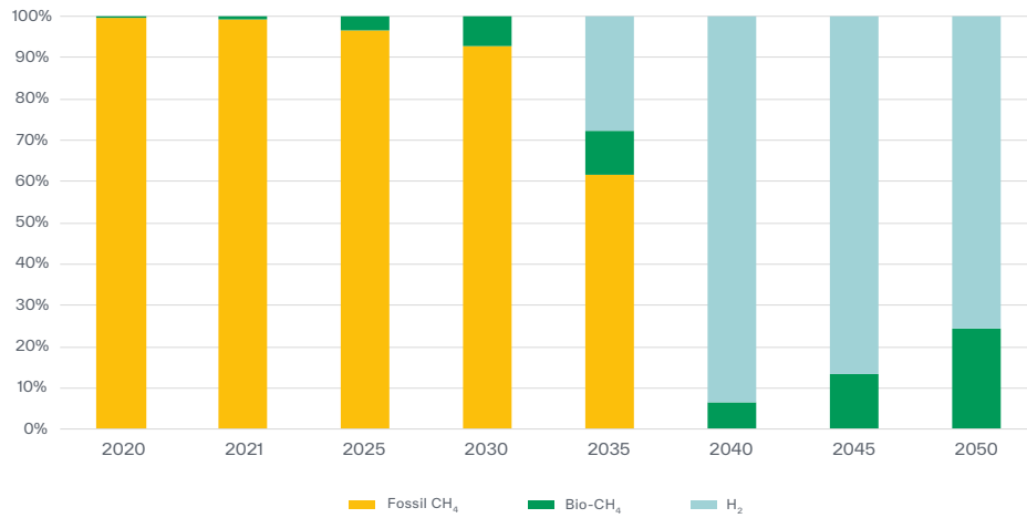
Figure 13: Calculated development of gas grid composition in ZEM after subtraction of gas for iron and steel and chemical and petrochemical industries.
